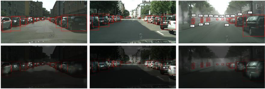
**Fig. 6.** Detection result on target domain. From left to right: Sim10k to Cityscapes; Kitti to Cityscapes; Cityscapes to FoggyCityscapes. The second row shows the weight inferred from our RPN weighted local domain discriminator. Brighter colors indicate higher attention. Apparently, regions with considered objects (e.g. car) are of higher weight in loss calculation. (Color figure online)
